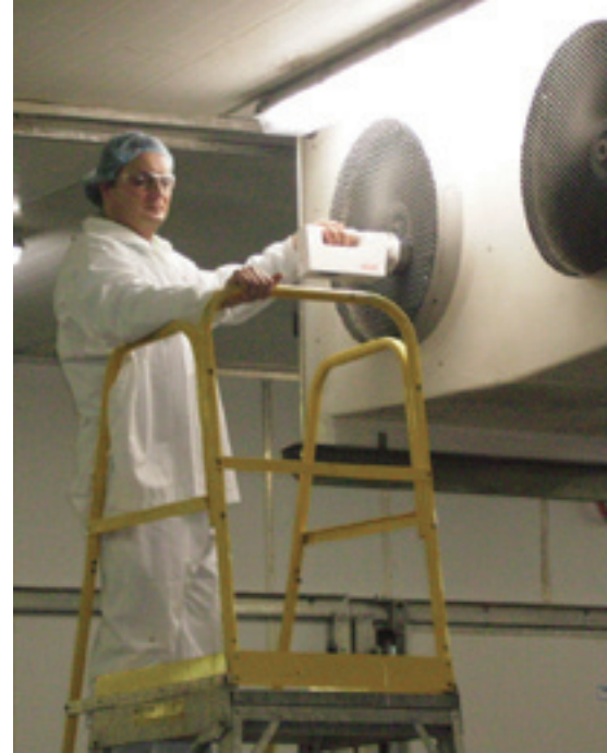
Measuring of germ load in and from no-frost-refrigerators.
