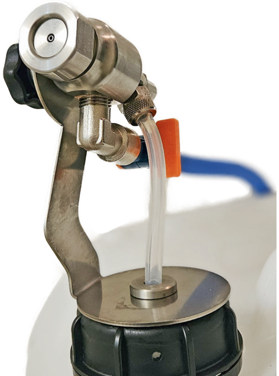
Fig. 1: For automatic disinfection, the ready-to-use solution is evenly atomised by a dual-component nozzle technology, which is mounted directly on ingredient canister.
