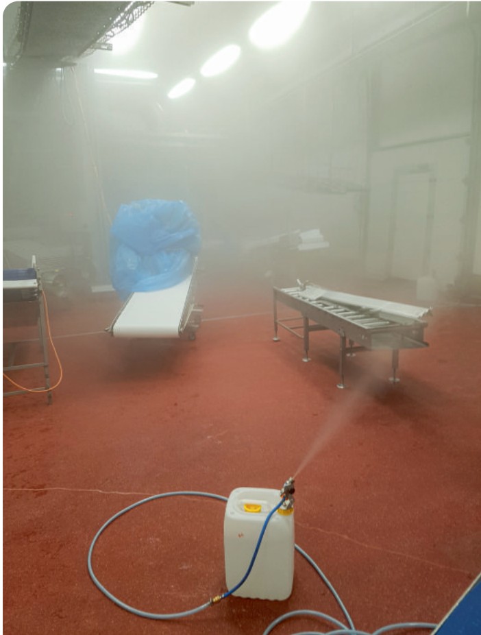
Abb. 4: All surfaces within the process area, ranging from product-contact components to installed peripheral equipment, are disinfected simultaneously. Photo: Just in Air GmbH
