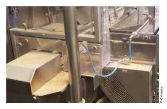
**\*\*** Accumulation of cutting dust from a slicing machine without suction exhaust
